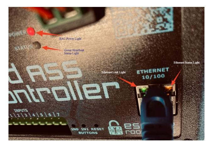
**Connecting your BAM to the network -** Copy the BAM from the SD card (or download from <u>https://www.escaperoomtechs.com/bad-ass-manager-software-p/e3001-001.htm</u>) to the Windows PC connected to IP network with DHCP. Click and run the BAM EXE software; the BAM software will open in a new tab on your default browser. On the home screen, click the Green Discover button to find the BAC. After a brief second, you will see the following basic BAC information on the Home screen:
